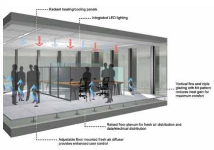
The radiant heating and cooling system and underfloor fresh air provides a highly efficient HVAC system. A high-performance envelope, building orientation and architectural details, such as triple glazing, and ceramic frit help control thermal gains and heat loss, and solar shading helps to reduce energy consumption.
