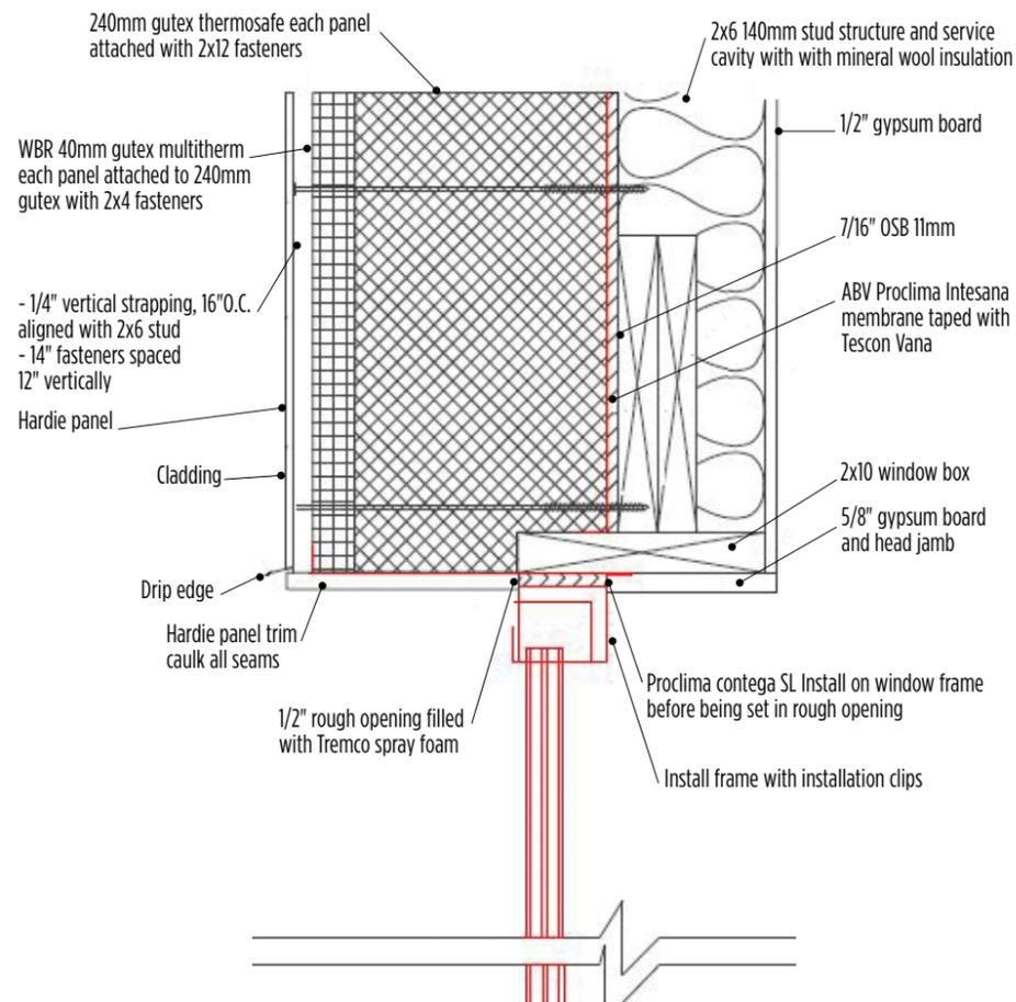
**Detail of the Radiance Co-Housing Project in Saskatoon, an example of a smart enclosure system**
